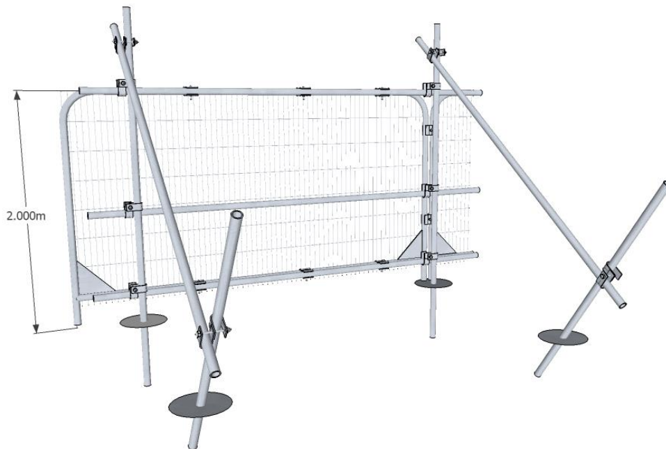
Figure 1. Protective fence specification
