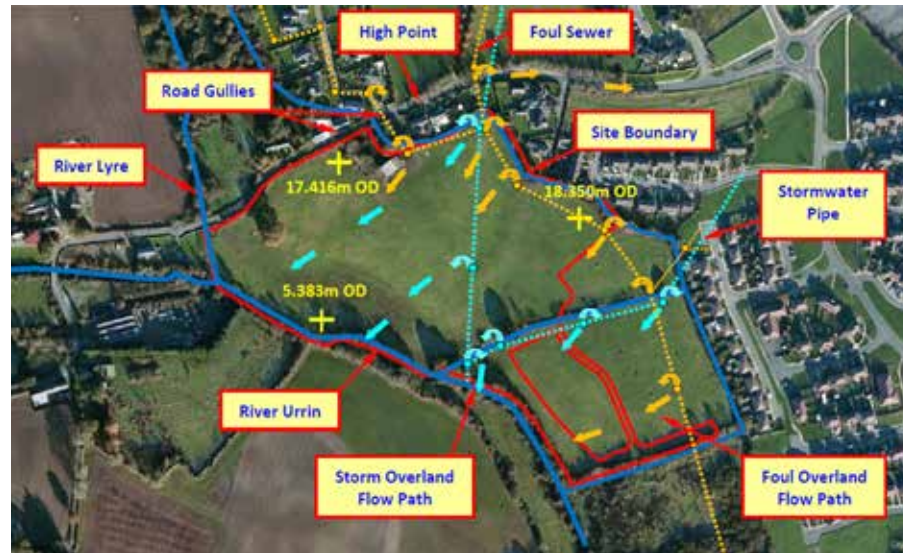
Above: By Consulting Engineer 'IE Consulting' - 'Overland Flow Paths'. Surface water flows across the site still follow the old field/drain boundaries, and provide a starting point for natural SuDS proposals.
