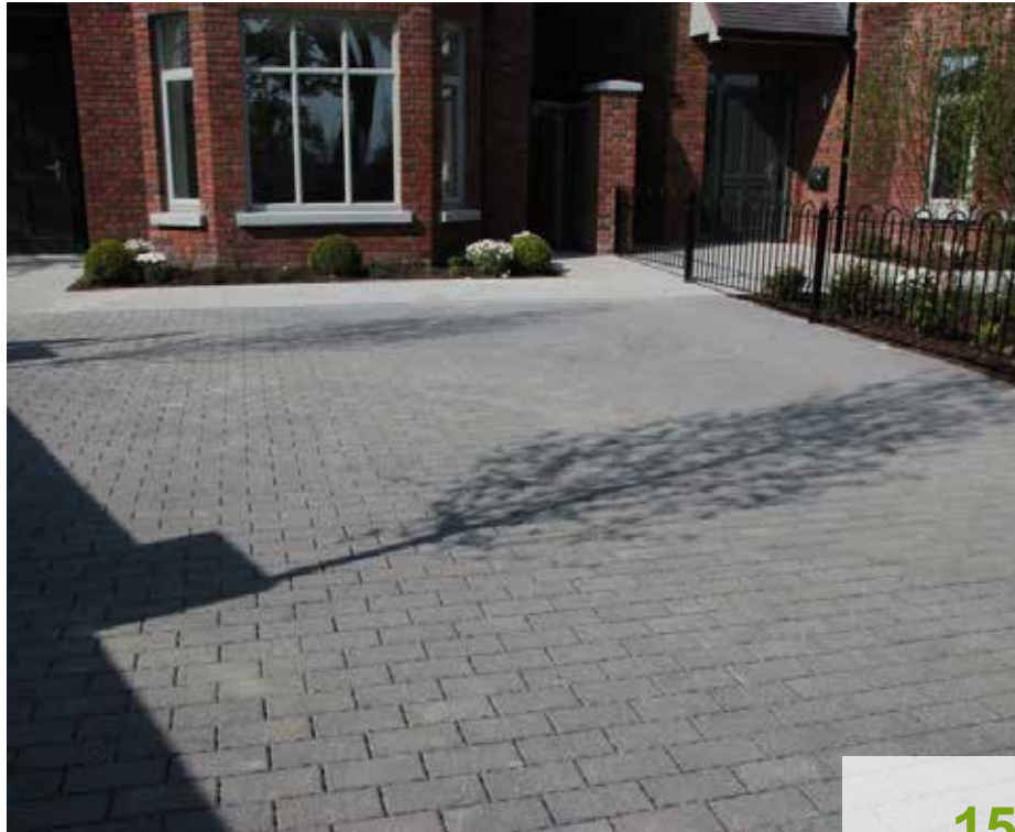
Above: permeable paving in 'Newgrange Clima-Pave' black ground granite aggregate finish, with 'Pembroke' silver grey granite paving to front entrance of dwelling
